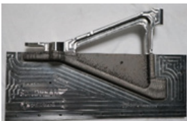
Pièce aéronautique imprimée pendant SoftDREAM Aeronautical part printed during SoftDREAM
